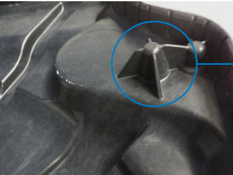
SMC vehicle floor pan with structural reinforcement material built up around traditional fixing solution
